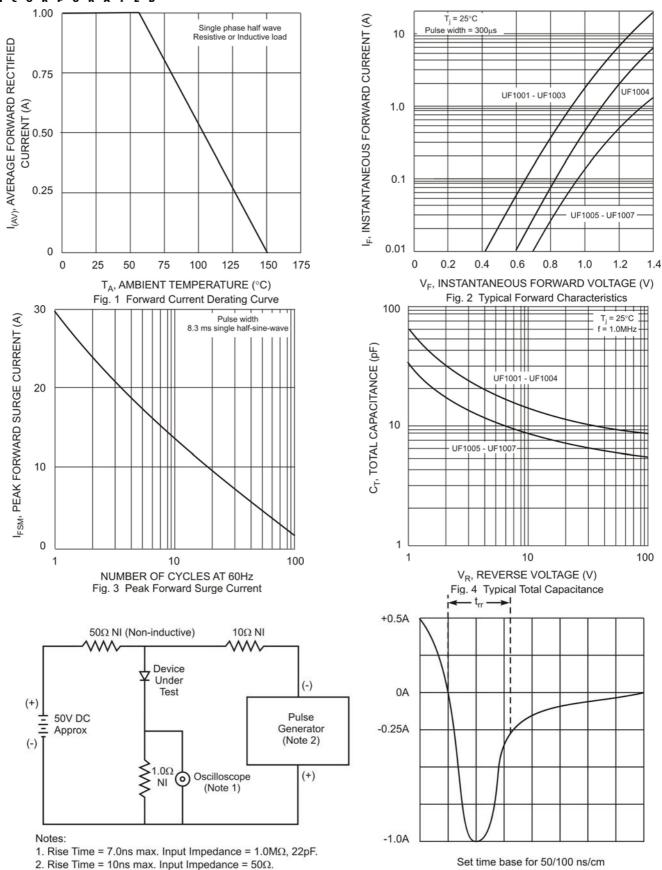
Fig. 5 Reverse Recovery Time Characteristic and Test Circuit
